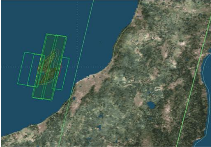
Figure 2. Beam selection to collect the highest value area for a SAR satellite
