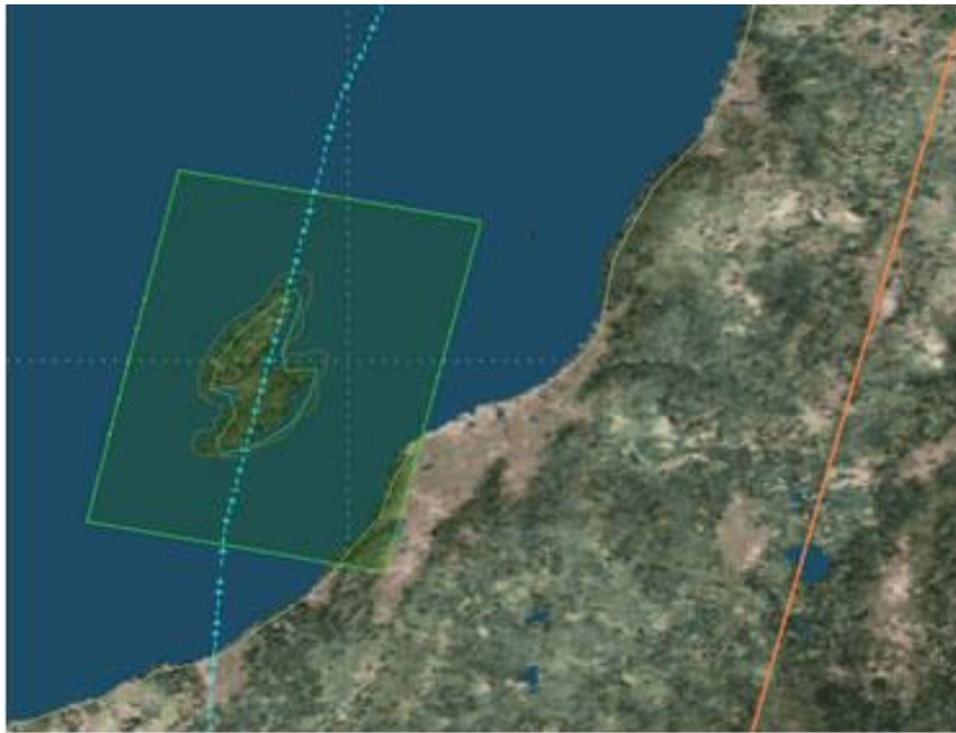
Figure 3. Slew and simple imagery collection for a low resolution Pushbroom satellite
